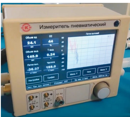
Fig. 4. View of the front panel of the Meter during the receipt of graphic and digital information
