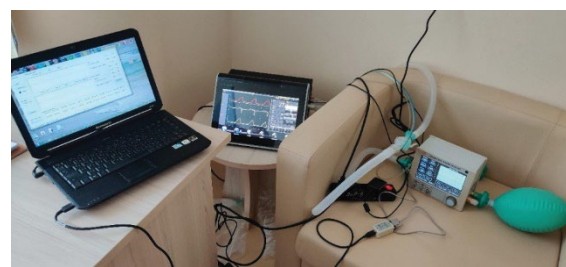
Fig. 2. Option for connecting the Meter to the ventilator circuit Note: Meter with test lung (right), Bellavista 950 ventilator (middle), laptop with developed Meter software (left)
