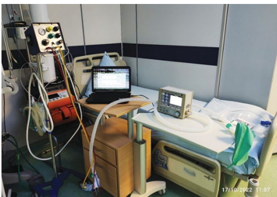
Fig. 3. Option for connecting the Meter to the Percussioner circuit: left — Percussioner; middle — laptop with software connected to the Meter; right — Meter with test lung
