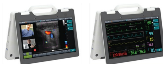
Fig. 3. Dialog window of the telemedicine complex during ultrasound examination with the possibility to comment on the resulting standard ultrasound image using markers of different colors (red and yellow) by each participant of the consultation, as well as the second tab of the window of monitored physical parameters from the patient
