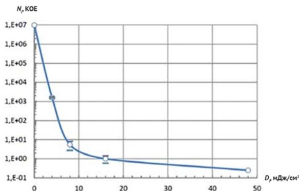
Fig. 2. The survival curve of *K. pneumoniae* bacteria under UV irradiation with an LED device. Horizontal shelves correspond to the standard deviation
