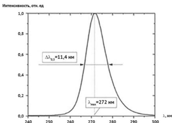
Fig. 1. Radiation spectrum of the device
