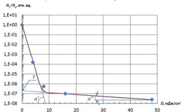
Fig. 3. Dependence of the relative number of surviving bacteria  $N_i/N_0$  on the dose. Squares are an experiment; a solid thick line is an approximation
