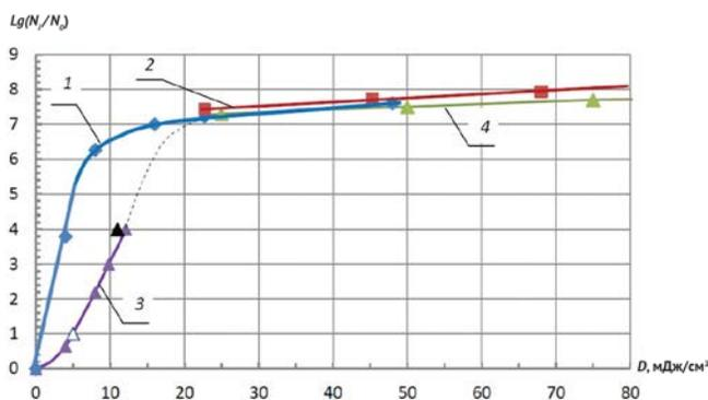
Fig. 4. Dependence of the logarithm of inactivation against *K. pneumoniae* bacteria on the energy dose of UV radiation. Squares – wavelength  $\lambda=272\pm 6$  nm; triangles – wavelength  $\lambda=254\pm 1$  nm.
